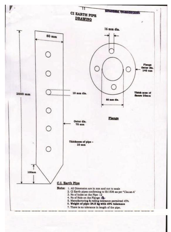
C.I Earth Pipes as per IS-1536/1976 Clause-A, 50mm Bore 2.00 meters long
